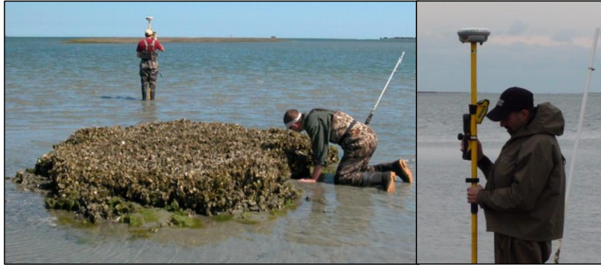
Figure 3. Left: Tony Rodriguez acquiring Trimble-based substate elevations while Joel Fodrie inspects a reef constructed by IMS graduate student Jon Grabowski in 1997. Right: Tony Rodriguez using the Trimble GPS system.
