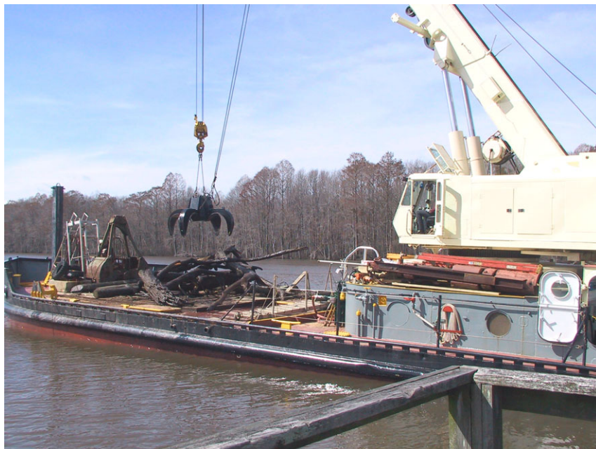
The USACE Snell removes woody debris, impacting in-stream habitat for substrate spawning anadromous fishes and for the resident aquatic community.
