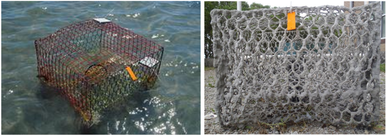
Figure 2. Examples of refurbished, recycled crab pots deployed as oyster settlement substrate. Note the removal of entrance funnels (both images) and addition of 1. Exit portal at top (left); 2. settlement plates (left), concrete coating (right), ID tags (both), and rebar anchor (left).
