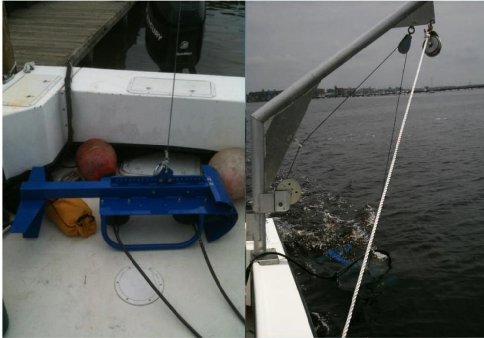
Figure 14. Photos of the SONAR (Biosonics DTX transducers on tow body, BioFin) and tow body being deployed at NR.
