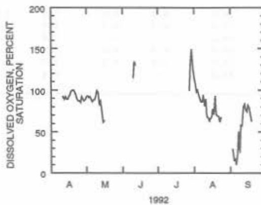
DAILY MEAN DISSOLVED OXYGEN, PERCENT SATURATION, NEAR BOTTOM, SITE 12, NEUSE RIVER AT LIGHT 7
