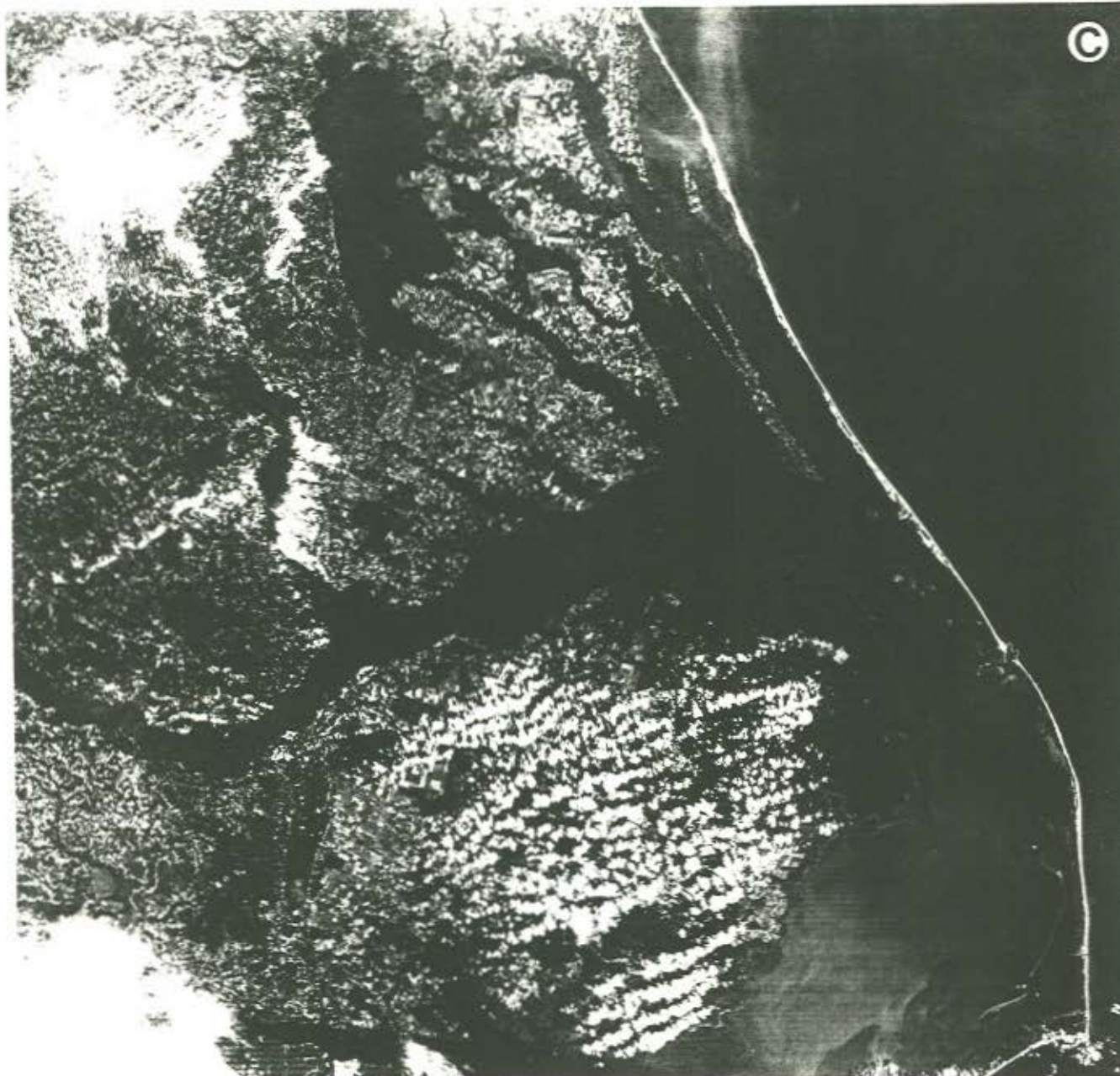
Figure 11C. Landsat Thematic Mapper image (Band 2) taken on October 7, 1984 showing the northern half of the APES region. High concentrations of suspended sediments are generally indicated by the high radiance values (white areas). Depth of penetration is dependent upon sediment concentration and actual values of turbidity cannot be determined without ground truth data at the time of satellite overpass. However, in shallow well mixed areas the bottom patterns may be similar to observed surface patterns. The fact that the open waters of Pamlico Sound have higher sediment concentrations than either Albemarle Sound or the tributary rivers suggests that wind-generated currents are the dominant process in resuspension, mixing, and advection.
