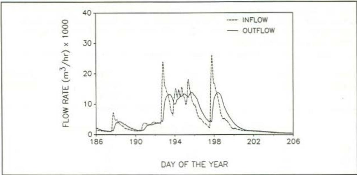
Figure 13. Inflow and outflow hydrograph for 2126 ha watershed section as predicted by FLDNSTRM. The II field design and the NC canal control level were used on the agricultural fields in the watershed. The simulation was conducted during a wet period in the summer (July, 1959).
