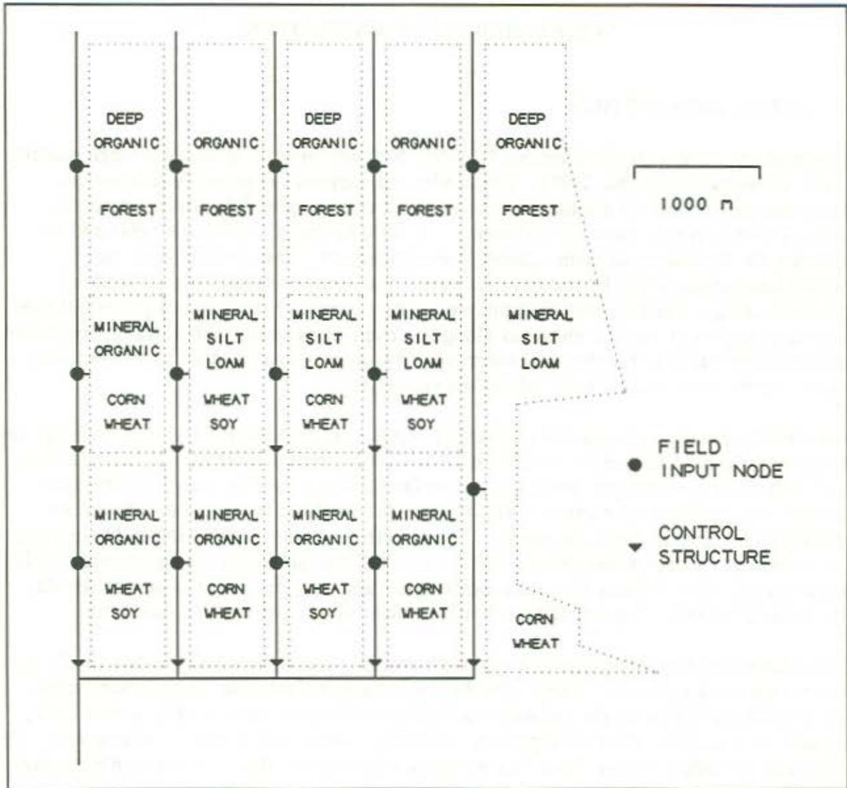
Figure 6. Discretization of watershed section used for the FLDNSTRM model.
