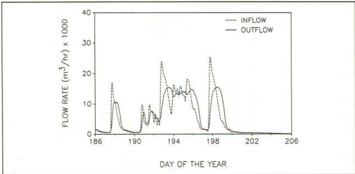
Figure 12. Inflow and outflow hydrograph for 2126 ha watershed section as predicted by FLDNSTRM. The UI field design and the HC canal control level were used on the agricultural fields in the watershed. The simulation was conducted during a wet period in the summer (July, 1959).
