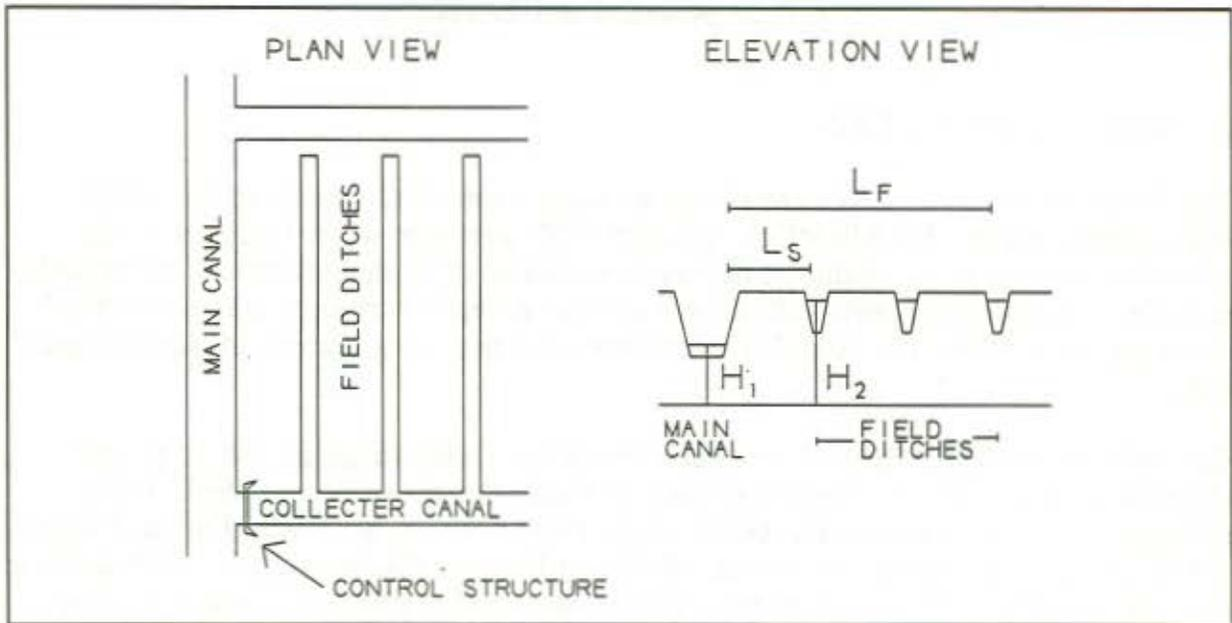
Figure 4. Schematic of canals and ditches on the fields of the watershed showing the variables used for calculating lateral seepage.
