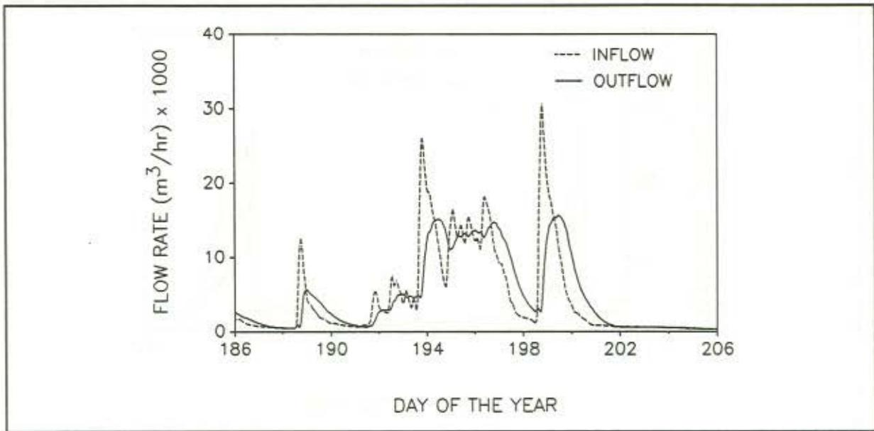
Figure 11. Inflow and outflow hydrograph for 2126 ha watershed section as predicted by FLDNSTRM. The UI field design and the NC canal control level were used on the agricultural fields in the watershed. The simulation was conducted during a wet period in the summer (July, 1959).
