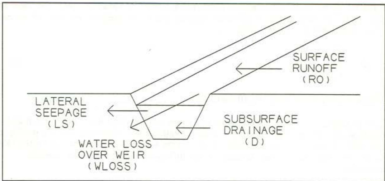
Figure 5. Schematic of variables in the water balance in the ditch (Eq 6).
