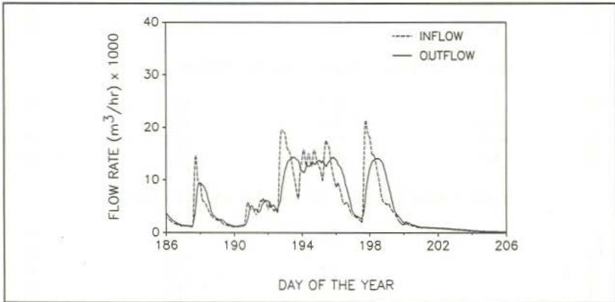
Figure 14. Inflow and outflow hydrograph for 2126 ha watershed section as predicted by FLDNSTRM. The II field design and the HC canal control level were used on the agricultural fields in the watershed. The simulation was conducted during a wet period in the summer (July, 1959).
