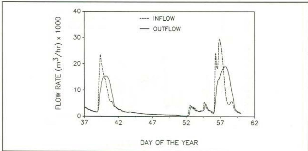
Figure 10. Inflow and outflow hydrograph for 2126 ha watershed section as predicted by FLDNSTRM. The II field design and the HC canal control level were used on the agricultural fields in the watershed. The simulation was conducted during a wet period in the winter (February, 1961).
