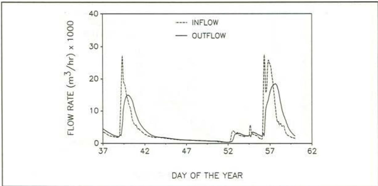
Figure 9. Inflow and outflow hydrograph for 2126 ha watershed section as predicted by FLDNSTRM. The II field design and the NC canal control level were used on the agricultural fields in the watershed. The simulation was conducted during a wet period in the winter (February, 1961).
