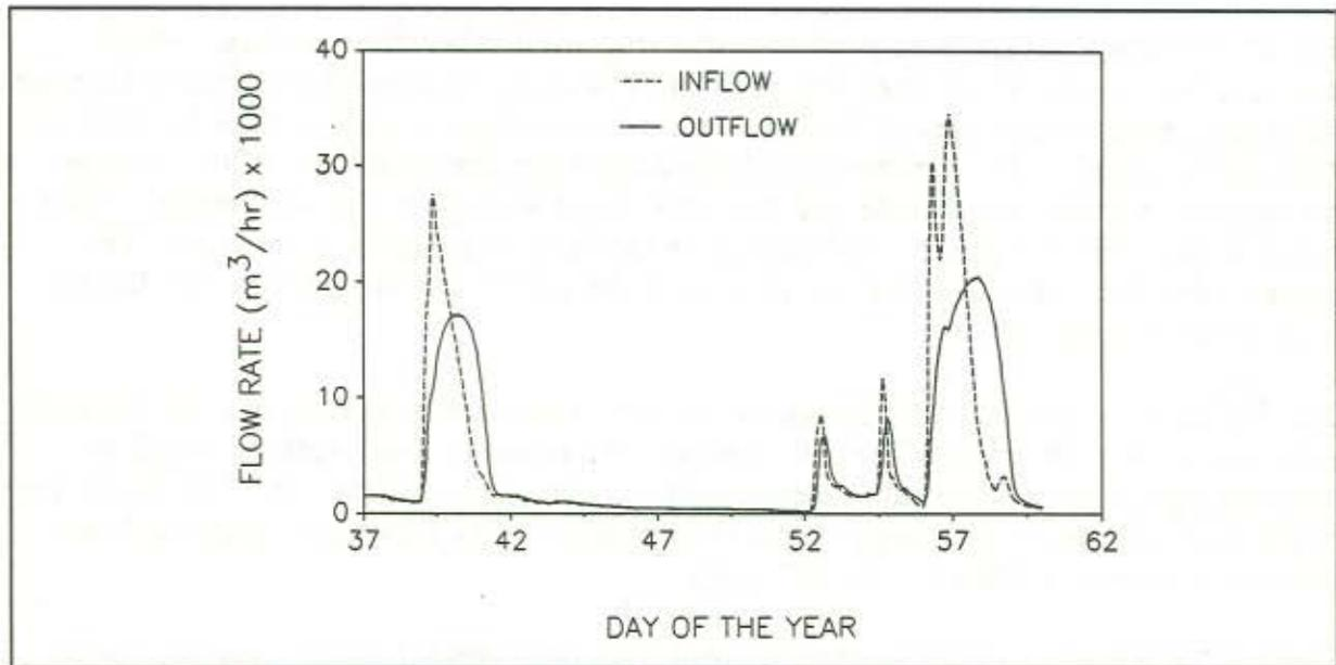
Figure 8. Inflow and outflow hydrograph for 2126 ha watershed section as predicted by FLDNSTRM. The UI field design and the HC canal control level were used on the agricultural fields in the watershed. The simulation was conducted during a wet period in the winter (February, 1961).
