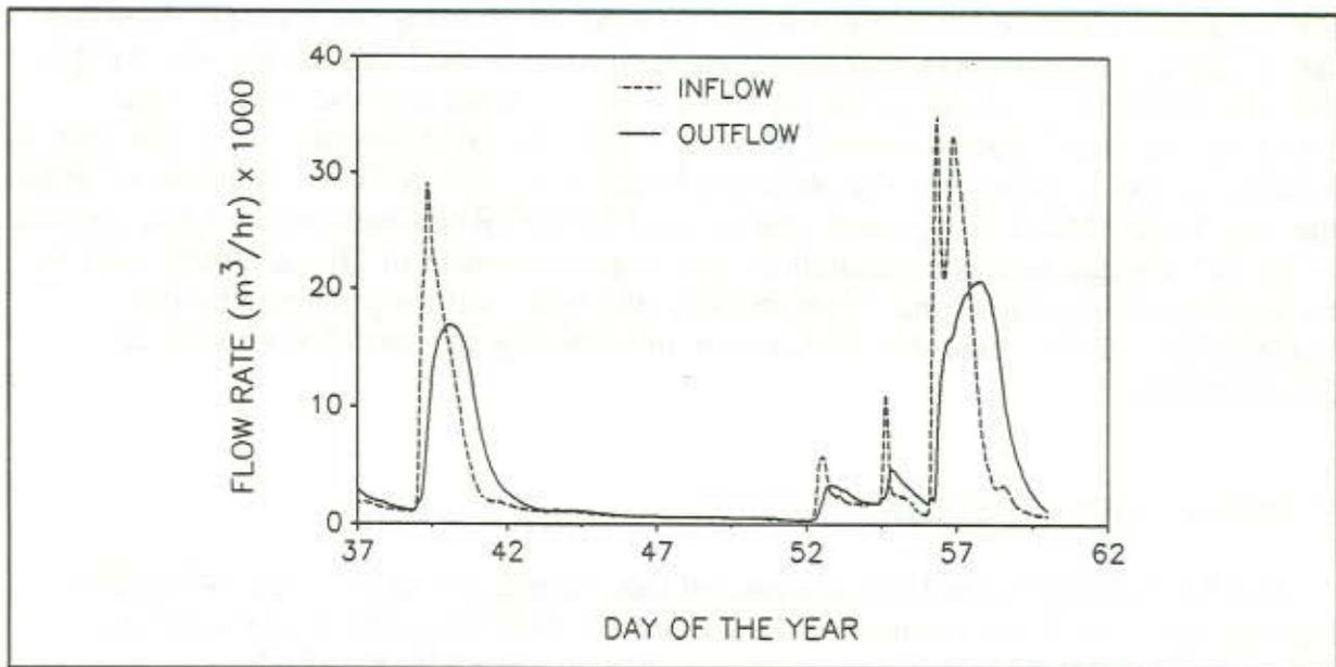
Figure 7. Inflow and outflow hydrograph for 2126 ha watershed section as predicted by FLDNSTRM. The UI field design and the NC canal control level were used on the agricultural fields in the watershed. The simulation was conducted during a wet period in the winter (February, 1961).
