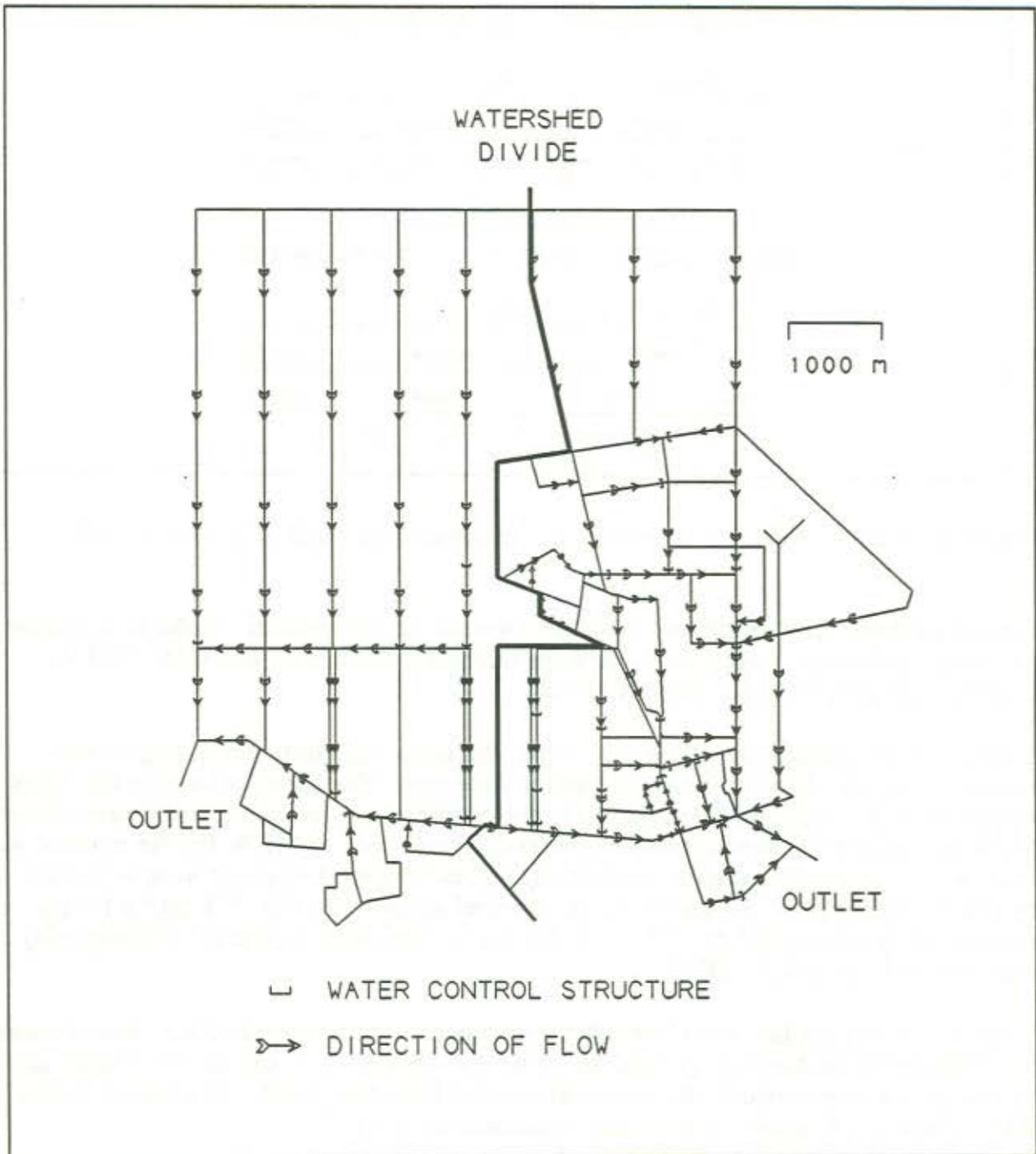
Figure 3. The network of canals on the watershed showing the flow directions and the location of canal control structures.
