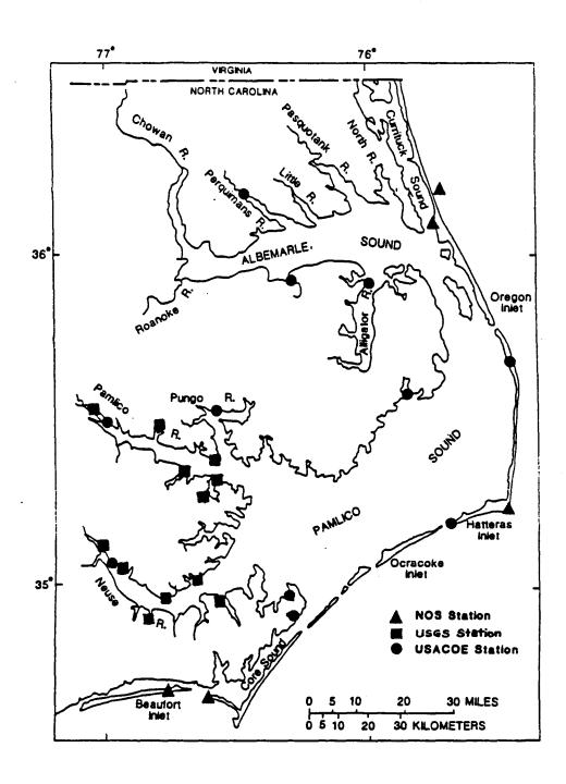
Fig. III-1. Tidal Elevation Gage Sites in the Albemarle-Pamlico Estuarine System, March 1989. From J.D. Bales, USGS, Personal Communication.
