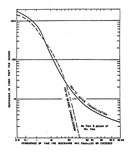
Fig. III-2. Flow Duration Curves for Ahoskie Creek at Ahoskie Before and After Channelization. From Winner and Simmons (1978).
